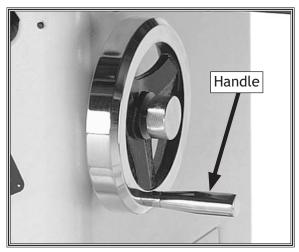
Figure 13. Handwheel handle installed.
